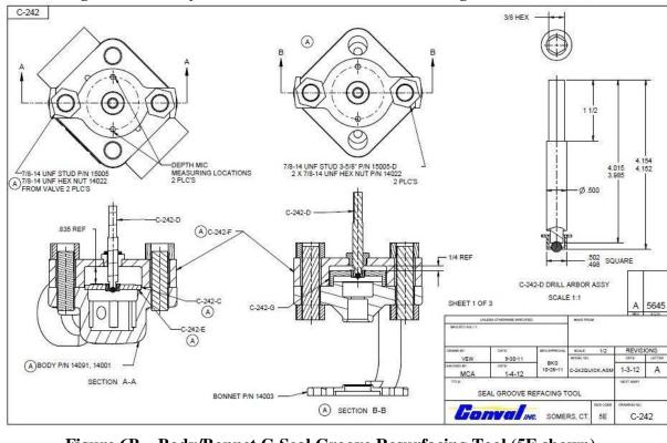
Figure 6A – Body/Bonnet C-Seal Groove Resurfacing Tool (5E shown)
