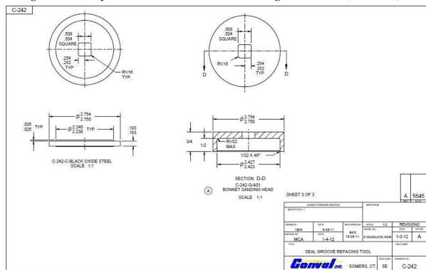
Figure 6C – Body/Bonnet C-Seal Groove Resurfacing Arbor Tools (5E shown)
